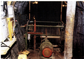
Photo 2. Rail vans winches
