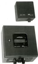
Photo 13. SMACH 2-SIG accelerograph
