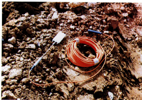
Photo 6. Total pressure cell
