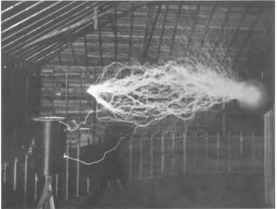
Phot. LVI. Discharge of "extra coil" issuing from a ball of 30" diam. forming the "free" terminal of the coil towards a coil on a stand.
