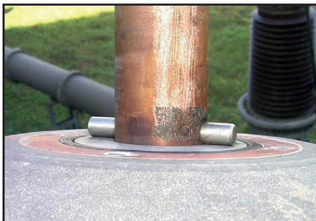
Figure 6: Left: Overheating traces on the HV connection and the tulip contact spring part; Right: Traces of overheating on the bolt
