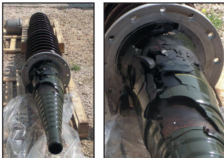
Figure 8 Burst of a 245 kV, RBP type, bushing, the upper porcelain envelope remained intact (left), detail of the burst lower part (right)
