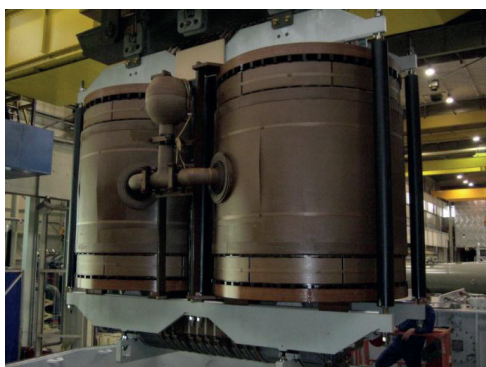
Picture 1 Active part in lifting crane before putting into tank
