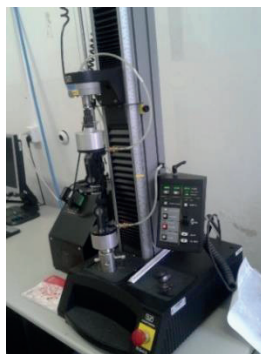
Figure 8: Testing equipment for EaB
