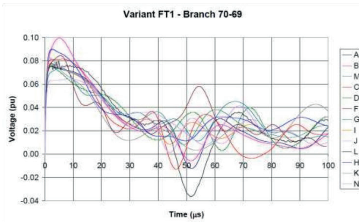
Figure 8: Voltage across the first discs of the HV winding from CIGRE brochure [1]
