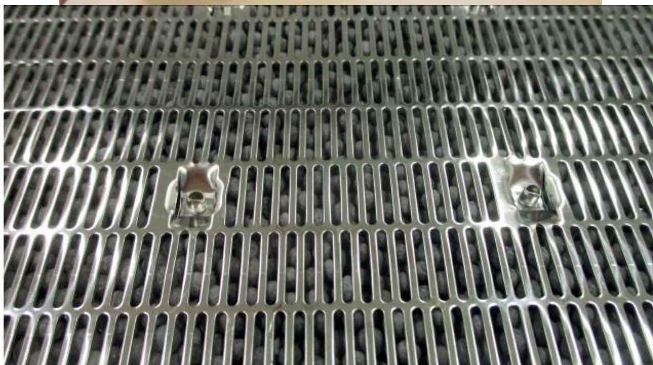
Figure 2: PAR cartridge with catalytic material
