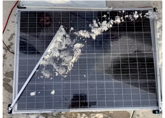
(b) Wiper system in action.
