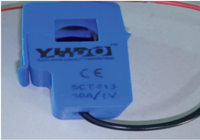
Fig. 4. SCT-013 Current Transformer
