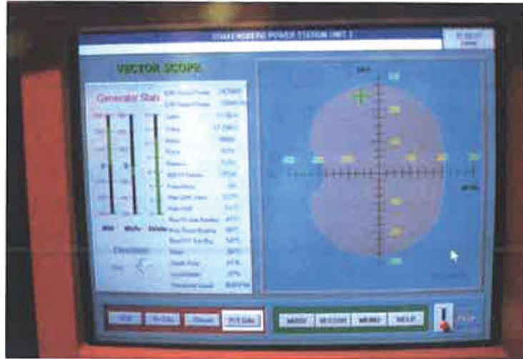
Drakenberg generator working point monitoring, photographed during a CIGRE Symposium in 1993 in South Africa
