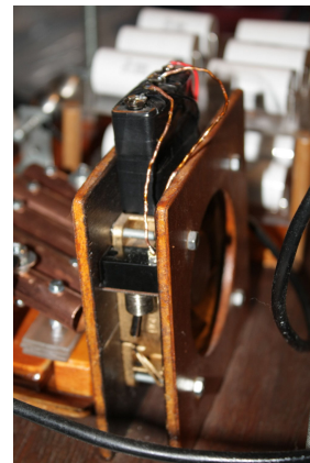
Figure 4.27: The power supply of the fan.
