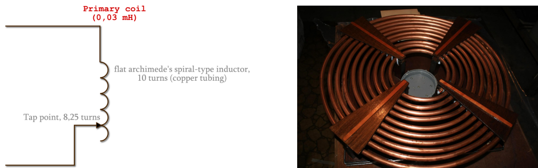
Figure 4.20: Schematic and photograph of Zeus' primary inductor (secondary circuit removed).
