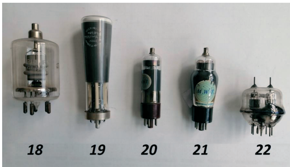
Sl. 6.: Philips QB3/300 (18), Philips – Miniwatt DG4-2 (19), MWT-KTW 61 (LC4) (20), MWT-KTW 61 (G) (21), RCA 832A (22)
