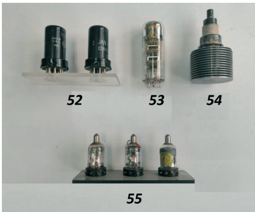
Sl. 14.: RCA JAN CRC – 12SK7 VT131 (52, lijevo), RCA JAN 12SR7 VT133 (52, desno), WF M10 FS301 (53), Siemens YD-1270 (54), Telefunken RV 12P 2000 – oznake Wehrmacht (55)
