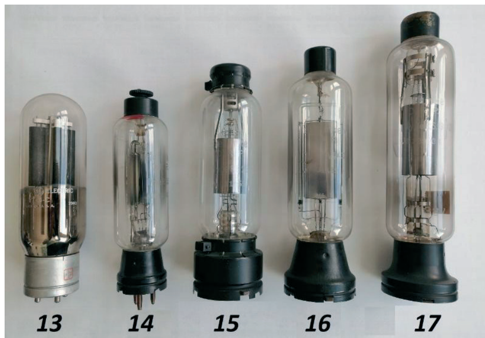
Sl. 5.: General Electric VT4c (13), Telefunken D.R.P. RS-59 (14), Telefunken D.R.P. RS-231 (15), Telefunken D.R.P. RS-24 (16), Telefunken D.R.P. RS-19 (17)
